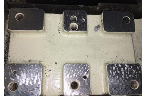
【State of the scraping on the mounting base of the tailstock】
