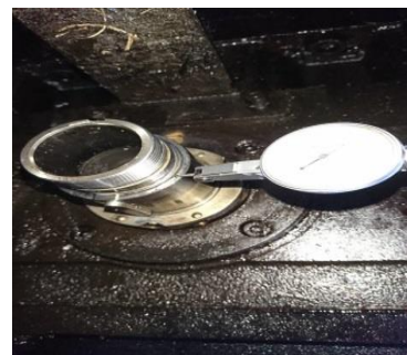
【Correct end face runout and outside diameter runout of cylinder mounting flange】
