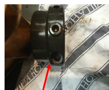
【Vibration due to missing bolts in mounting parts】
