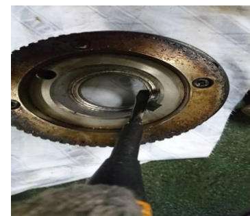
【Correct end face runout and outside diameter runout of cylinder mounting flange】
